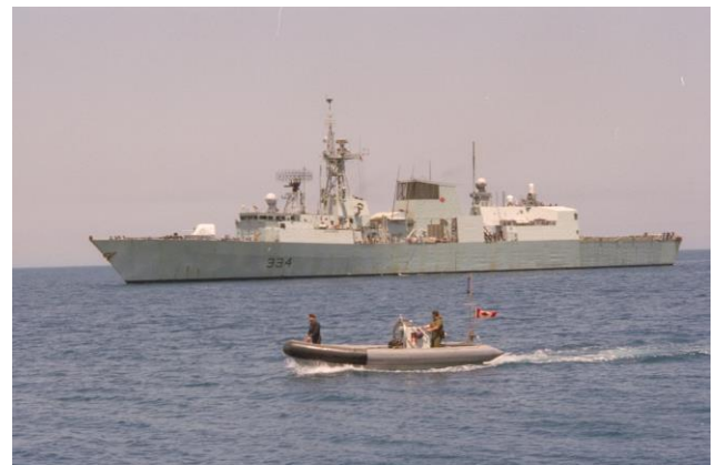
▲ HMCS Regina with its Rigid-Hull Inflatable Boat used for boarding operations in the foreground.
